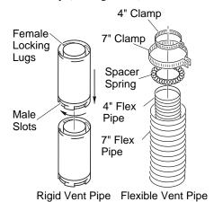
Figure 11 - Vent Pipe Connections
